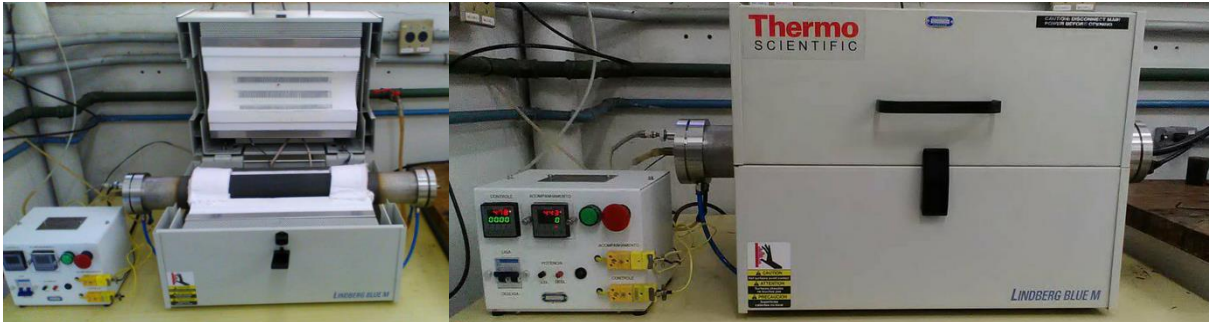
Figura 7: Imagens do reator de pirólise (Thermo Scientific Lindberg, modelo Blue M 1100C Tube Furnace).
